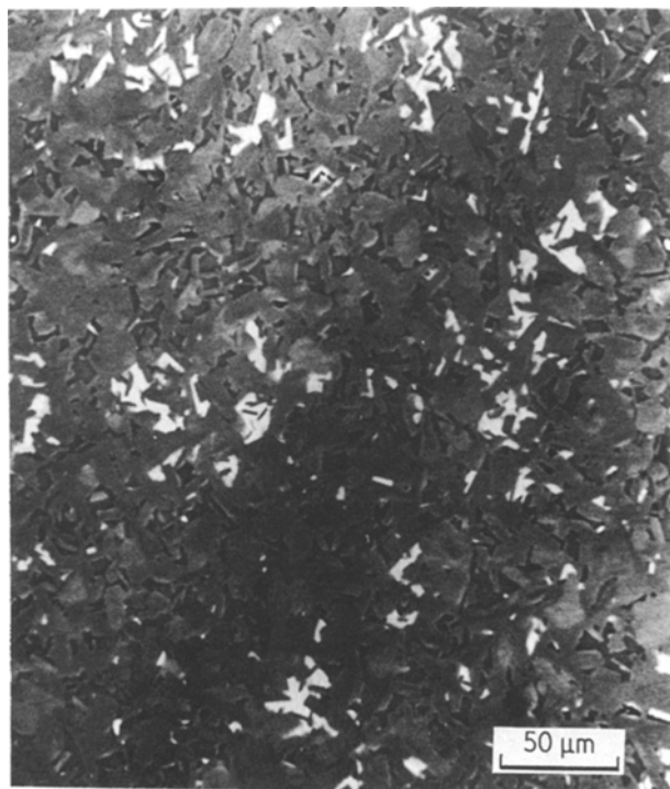
Figure 6 Scanning electron micrograph of a dense SiC body prepared at 2150°C from 75 wt% SiC, 10 wt% additive A (4.3 wt% Al 2 O 3 ) and 15 wt% additive Y (8.1 wt% Y 2 O 3 ).
